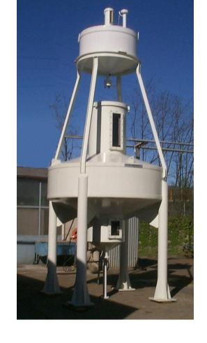
Calibration is made by filling the proving tanks by using smaller volume tanks (1000 or 2000 litres), often mounted on the proving tanks to be calibrated in order to make tests easier and faster.
