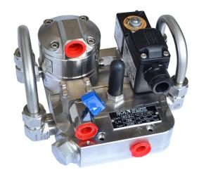
The IB2 is a compact metering group that carries out precise additive injection.
