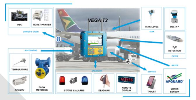
Thanks to its extended communication features (serial lines, Ethernet port, Bluetooth compatible peripheral and WiFi), VEGA T2 can make all the measure and automation information available to remote units such as on board computer or external devices for data acquisition and transmission. At the same time VEGA T2 drives a ticket printer directly, with legally relevant functions.
