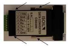
Open the module by levering the points indicated by the arrows with a screwdriver.
