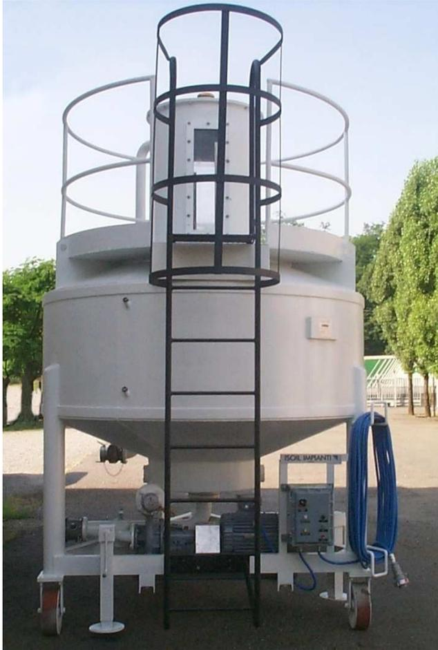
Proving tanks are used as a primary provers to calibrate p.d.meters, dosing pumps or analogous proving tanks on secondary lines. They can be trucked on-side to monitor meters installed in loading bays or in different places in the refinery.
